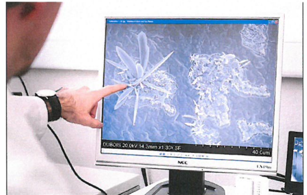
Silver sulphide needles on the surface of a dial.
