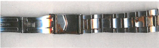
Salt spray test on watch cases.
