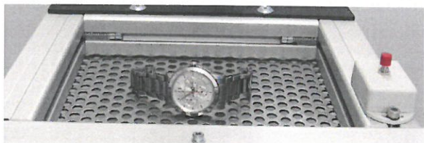
Free fall test on a complete watch
